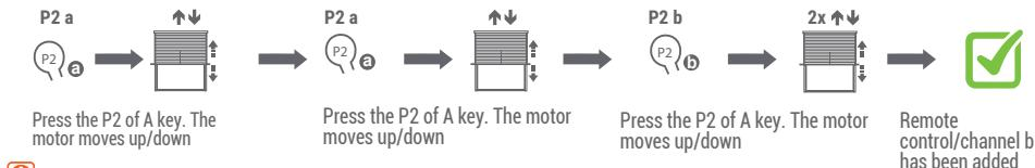
**Start with the transmitter or channel that the motor is programmed to**
