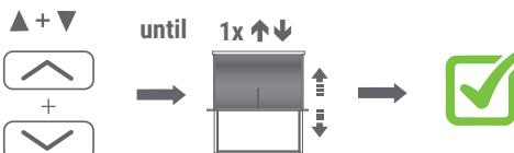
Press the UP and DOWN buttons simultaneously until the motor moves up/down.
