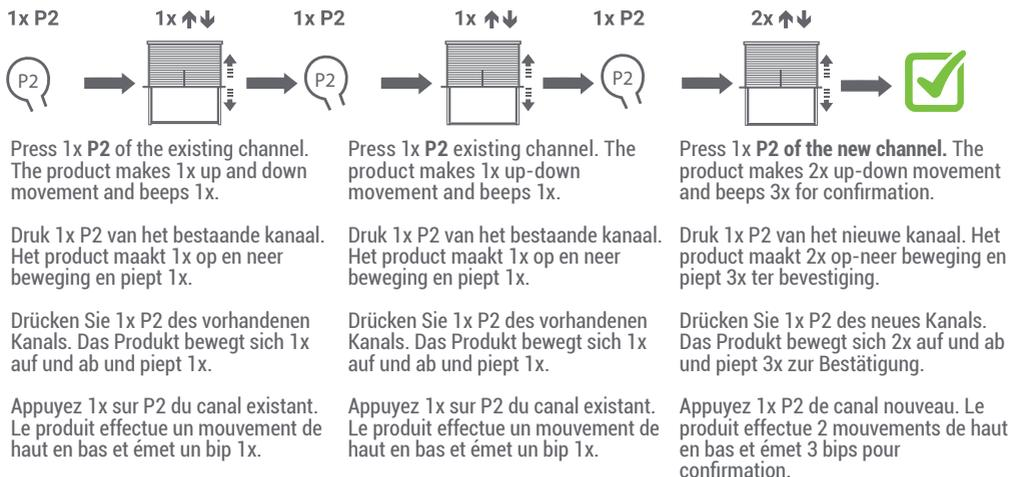
Press 1x P2 of the existing channel. The product makes 1x up and down movement and beeps 1x.
