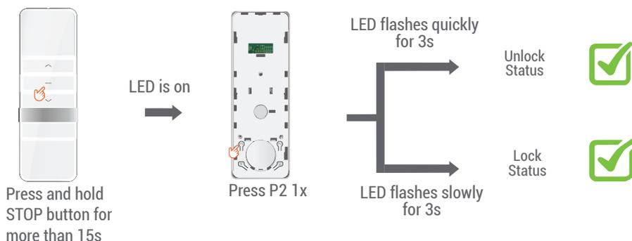
**NOTE** With the lock function you can not program functions in which you need two buttons like limit settings and change direction.
