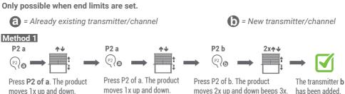
Make sure the new transmitter is in the desired channel.
